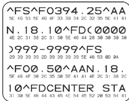
Figure 4 Communications Diagnostics Test Label
