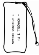
Rechargeable Li-ion battery pack (installed)
